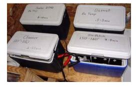
Plastic Coolers, buckets, storage containers all work well for setting up an anodizing line.
