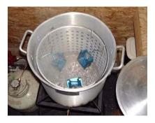
The best way to seal the part is to use a Nickel Acetate sealer. It produces a better quality surface then using heat. This sealer comes with most anodizing kits. I use a room temperature sealer of this type. Just place the dyed part in the room temperature bath for 5-10 minutes, then rinse and hang to dry for about 10 hours. No heat needed and the quality is great! There are some nickel acetate sealers that require some heat, but again, the surface quality is much improved when using Nickel
