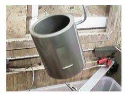
Notice the color of the anodized part. It should have a pale lemon tint if it is a 6000 series alloy, or a chalky white look for other types of aluminum alloy. Don't pull it out of the tank until it changes color. The following photo shows the color of 3 samples - natural aluminum, anodized, and dyed black.
