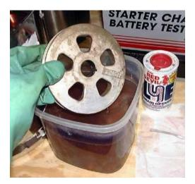
When the part is completely uniform (no remaining spots), rinse it off and buff it back to a shine. Stripping aluminum this way will create a matte finish. Polishing it back to its original surface is up to you. At this point, the part can be re-anodized and dyed any color just like a freshly machined part. Note: if the aluminum part has other metal steel parts pressed into it, do not re-anodize the part. Metals other than aluminum will dissolve away during the anodizing process.
