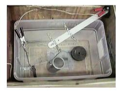
Bubbles will start foaming off both the cathodes and the part. I would advise not breathing the fumes, and would suggest some way of venting them away from your work area. I put the plastic tank in a sealed wooden box with a fan to vent the fumes out a nearby window using a simple dryer hose. Some anodizing kits provide fume control balls that take care of the problem. I have not tried them, but hear they work well.
