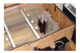
6061 aluminum is used as cathodes in this configuration. It is recommended that the cathodes should be removed when not in use, however I don't bother. The aluminum ones here are turning black after about 4 months in the acid without being removed. The lead ones were in the acid for more than 4 years!
