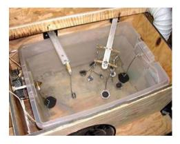
This configuration was one I used for small parts years' ago. It used small lead cathodes wired to the negative side of the battery charger using aluminum wire. Note the alligator clips for hanging the parts.
