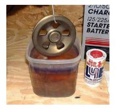
The lye will dissolve the old anodized layer, about .0005" thick. It takes a while for it to start breaking through the layer. It's a little slow at first. The first ten minutes or so not much action will be seen. Bubbles and smut will rise up as an indicator of its progress.
