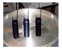
Note the middle part failed to take the black dye due to not being fully anodized. The electrical connection was at fault. The part was returned to the anodizing tank BEFORE sealing. It was then anodized fully after fixing the connection and re-dyed.
