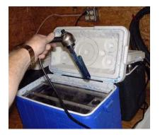
Here is a 5-gallon blue dye tank with the heater pulled out and hanging rack installed. You can simply use a plastic container and microwave it to heat up the dye if needed. It does not have to be anything fancy.
