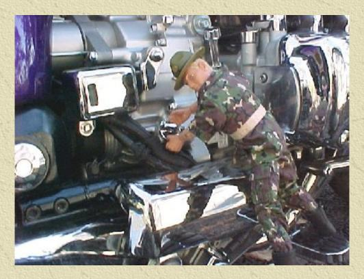
Now locate and remove the oil filler cap on the right side of the engine.....
