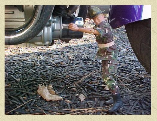
And install the new filter on the bike turning clockwise until the gasket seats snug against the mount, then turn the filter 1/4 turn more. The filter should be tight at this point. If you can still turn it without much effort you did it wrong...SO DROP AND START PUSHING YOUR WAY TO CHINA!!!!
