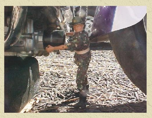
Now move up to the oil filter located on the front of the engine directly behind the front fender .If you have a strong grip you can grasp the filter and twist counter clockwise to loosen it. DID I SAY REMOVE IT PRIVATE? NO! NOW CLEAN THAT OIL UP!
