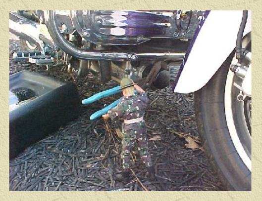
If you can't loosen the filter use a filter wrench or a pair of channel locks to do the job...DONT crush the filter with the channel locks.
