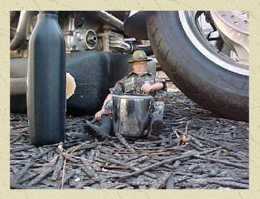
Now apply a light coat of clean oil to the gasket on the new filter.....
