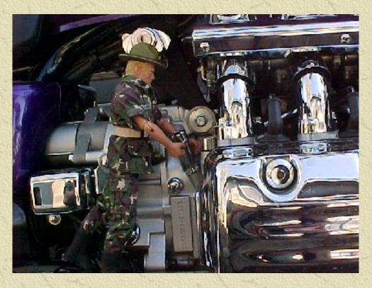
Locate and remove the dipstick, wipe it off, and with the bike upright re-insert it into the hole without screwing it in.
