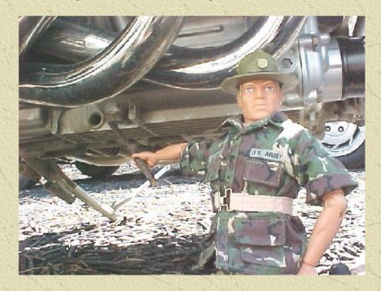
The first thing we need to do is place the F6-C on it's side-stand on a firm surface and locate the drain plug on the bottom right side of the engine.
