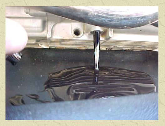
Now let the oil drain into the pan.....when it stops draining stand the bike upright so any residual oil can drain. Now replace the bolt and **tighten** with the 17mm box wrench. wipe up and spilled oil around the bolt.
