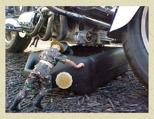
Now move the oil pan under the filter, remove the filter and allow it to drain into the pan. Then wipe off the filter mount on the bike.
