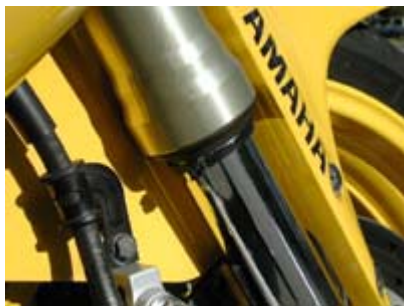
You Need to Push the Zip Tie Against the Fork Seal with the Rider Sitting On the Bike in Full Riding Kit
