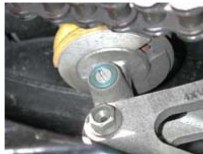
Rear Rebound Adjuster Hint: Look Under the Chain Side of the Rear Shock
