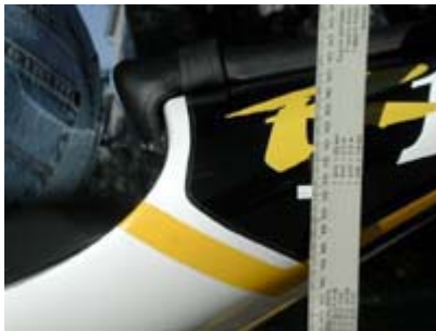
This Shows Rear Sag At 53.5mm Compressed. (Rider on board Wearing Full Riding Kit)
