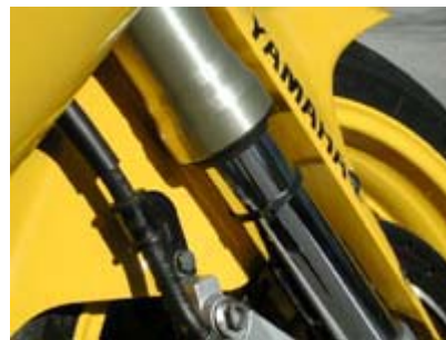
This Shows the Difference between the Sag with a Rider on Board and Then With Suspension Pulled Up, it Should be 30mm
