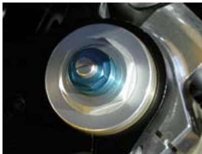
Top of Fork Leg Showing the Blue Preload Adjuster and the Rebound Screw on Top in the Middle
