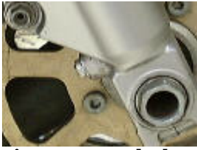
Projecting screw on the bottom of the fork leg adjusts compression
