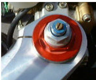
The little screw does the rebound and the silver nut does spring preload
