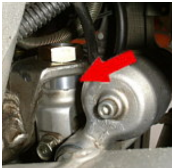
Use a suitable spacer to increase rear ride height
