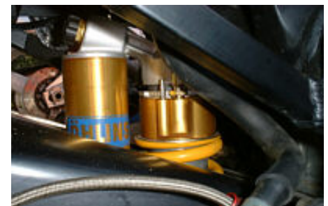
Knurled knob at top adjusts compression on rear shock
