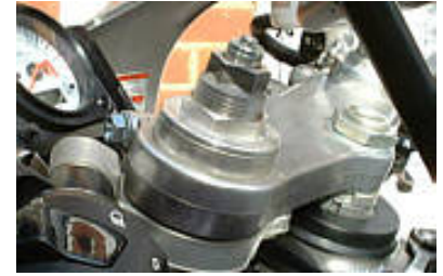
Raise the forks through the yokes to drop the front end
