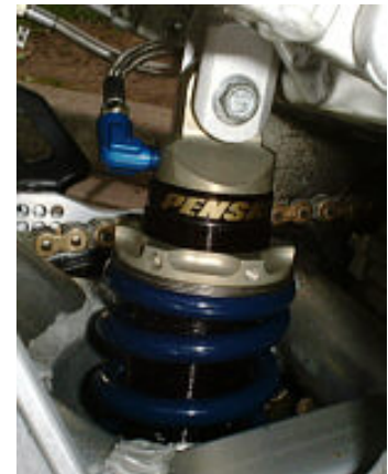
Alloy collar above spring screws down to increase preload
