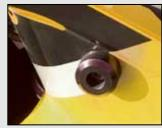
motorcycle frame and save expensive fairing bits—and levers, pegs, turn signals, mirrors, anything else that sticks out—from being fouled in a tip-over or crash. Plenty of colors, shapes and sizes are available (even some that light up!), and every last one is cheaper than even one piece of OEM plastic.
