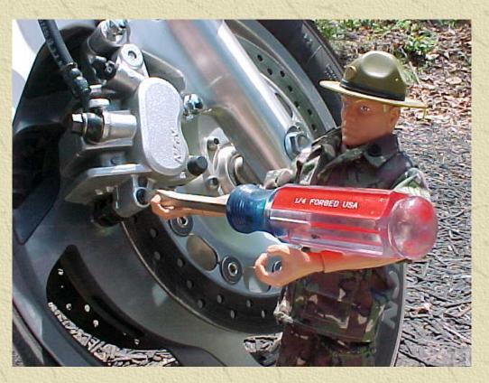
First use the screwdriver to remove the gunmetal gray plug on the lower portion of the caliper, This will expose an allen (hex) head bolt underneath.
