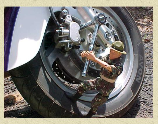
Next use the ratchet extension and 12mm socket to loosen the 2 chrome bolts holding the caliper onto the mount.
