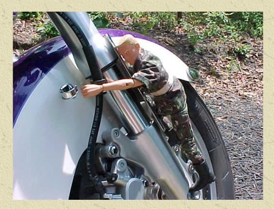
Pop the brake line from it's retainer and drape the towel over the fender to keep the caliper from scratching it.
