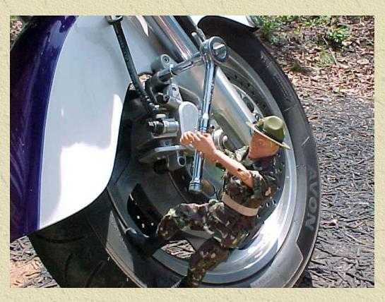
Remove the 2 chrome retaining bolts and turn the caliper so you can look at the pads.
