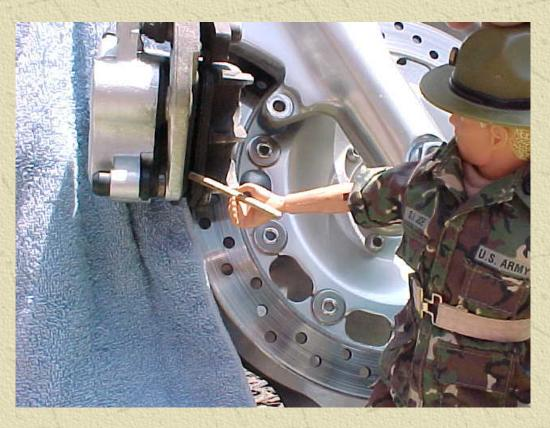
Observe how they are attached to the caliper. The top of the pad is inserted into a groove in the top of the caliper and a bolt runs through a hole in the bottom of the pad. Now use the allen head wrench to remove the bolt you loosened earlier and remove the pads.
